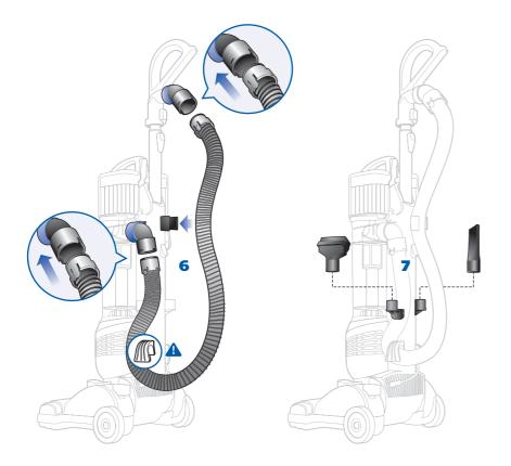
6 Attach each end of the Super Stretch Hose to the vacuum and press into Upper Hose Holder for easy storage.
